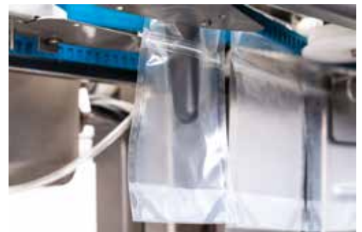
Shown: Stand-Up pouches with zipper on a FAS SPrint Revolution SidePouch System
